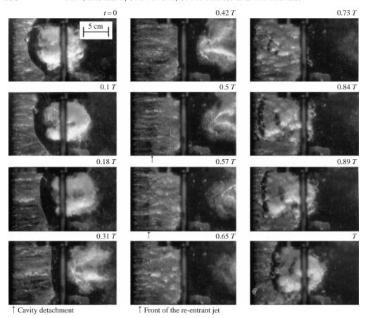
FIGURE 9. Visualization of the re-entrant jet and of the cavity auto-oscillations (cloud cavitation). Flow velocity  $11.6\,\mathrm{m\,s^{-1}}$ , confinement height  $e=20\,\mathrm{mm}$ , step height  $h=3.6\,\mathrm{mm}$ , divergence angle  $4.2^\circ$ . The period of the oscillation is 35 ms. The flow is from left to right.
