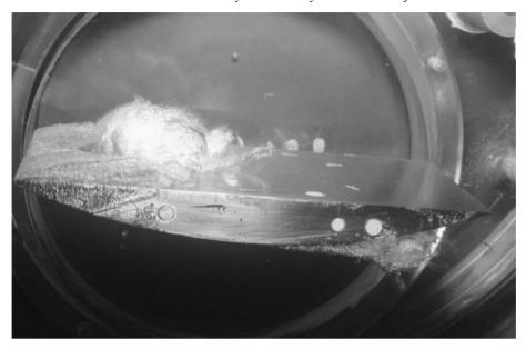
FIGURE 4. Typical view of the re-entrant jet instability and associated cloud cavitation on a plano-convex hydrofoil (angle of attack 3°, cavitation number 0.54, Reynolds number  $2 \times 10^6$ , maximum cavity length  $\approx 72$  mm, flow is from left to right).
