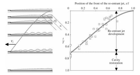
FIGURE 12. Evolution of the cavity and the re-entrant jet in the case of a thin cavity with a re-entrant jet (domain 2 of figure 8). Flow velocity  $11.6 \,\mathrm{m\,s^{-1}}$ , confinement height  $e=20 \,\mathrm{mm}$ , divergence angle  $\alpha=4.2^\circ$ , step height  $h=0.8 \,\mathrm{mm}$ , cavitation number  $\sigma=3.2$ , Cavity length  $l=100 \,\mathrm{mm}$ , period of the re-entrant jet  $T=38 \,\mathrm{ms}$ .
