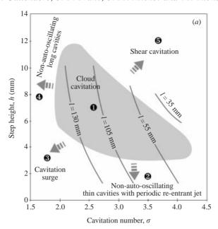
FIGURE 8. Mapping of the cloud cavitation instability and surrounding cavitation regimes for a flow velocity of  $11.6\,\mathrm{m\,s^{-1}}$ , a confinement height  $e=20\,\mathrm{mm}$  and a divergence angle of  $4.2^\circ$ . (a) obtained from direct observation of cavitation patterns under stroboscopic lighting; (b) obtained from velocity fluctuation measurements.
