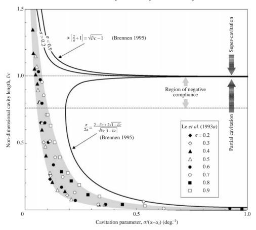
FIGURE 1. Typical variation of the cavity length l with the cavitation number  $\sigma$ . The cavity length l is made non-dimensional by the chord length c of the foil and the cavitation number is divided by the difference between the angle of attack  $\alpha$  and the incipient angle of attack  $\alpha_i$ . As a reference, the linear solution for a flat-plate hydrofoil (Brennen 1995) is shown in solid line.
