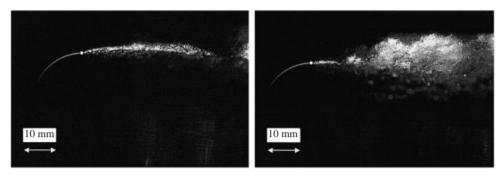
FIGURE 18. Instantaneous visualizations of the cavity interface by a laser sheet. Case of an auto-oscillating cavity at two different instants in the cycle (cloud cavitation). Flow velocity  $11.6\,\mathrm{m\,s^{-1}}$ , confinement height  $e=20\,\mathrm{mm}$ , divergence angle  $\alpha=4.2^\circ$ , cavitation number  $\sigma=3.2$ , step height  $h=4\,\mathrm{mm}$ . The flow is from left to right. The duration of the light sheet is  $20\,\mathrm{ns}$ .
