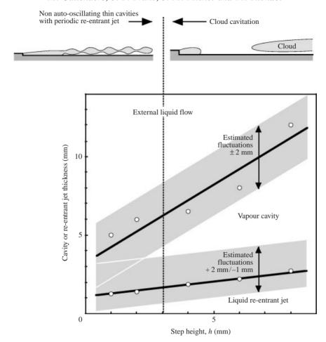
FIGURE 17. Evolution of the thicknesses of the re-entrant jet and of the cavity as a function of the step height. Flow velocity  $11.6 \,\mathrm{m\,s^{-1}}$ , confinement height  $e=20 \,\mathrm{mm}$ , divergence angle  $\alpha=4.2^\circ$ , maximum cavity length  $l=95 \,\mathrm{mm}$ .
