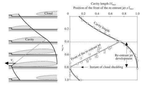
FIGURE 11. Evolution of the cavity and the re-entrant jet in the case of the cloud cavitation instability (domain 1 of figure 8). Flow velocity  $11.6\,\mathrm{m\,s^{-1}}$ , confinement height  $e=20\,\mathrm{mm}$ , divergence angle  $\alpha=4.2^\circ$ , step height  $h=3.6\,\mathrm{mm}$ , cavitation number  $\sigma=3.2$ , maximum cavity length  $l_{max}=100\,\mathrm{mm}$ , period of oscillation  $T=35\,\mathrm{ms}$ , Strouhal number S=0.25.
