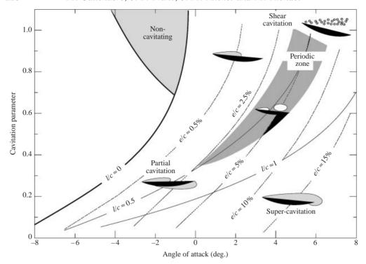
FIGURE 3. Cavitation patterns on the upper side of a plano-convex hydrofoil (after Le *et al.* 1993a). The periodic zone corresponds to the presence of a re-entrant jet and the develoment of cloud cavitation. l/c and e/c are the cavity length and the cavity thickness, non-dimensionalized by the chord length. In the case of cavity pulsations, l is the maximum cavity length.
