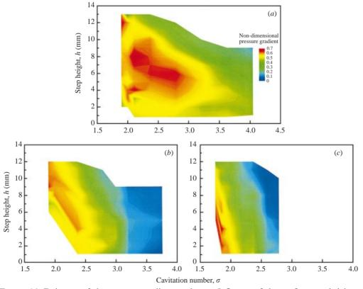
FIGURE 14. Estimates of the pressure gradient at closure. Influence of the confinement height at divergence angle 4.2°. The pressure gradient is non-dimensionalized by the cavity length. (a) Flow velocity  $11.6\,\mathrm{m\,s^{-1}}$ , confinement height  $20\,\mathrm{mm}$ , (b) flow velocity  $9.6\,\mathrm{m\,s^{-1}}$ , confinement height  $40\,\mathrm{mm}$ ; (c) flow velocity  $8.5\,\mathrm{m\,s^{-1}}$ , confinement height  $60\,\mathrm{mm}$ .
