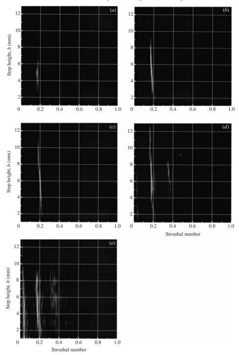
FIGURE 19. Spectra of the pressure transducer fluctuations for various operating conditions. The spectra obtained for various step heights are juxtaposed. Flow velocity  $11.6 \,\mathrm{m\,s^{-1}}$ , confinement height 20 mm, angle of attack  $4.2^{\circ}$ . Each diagram corresponds to a given cavity length: (a) 50 mm, (b) 75 mm, (c)  $100 \,\mathrm{mm}$ , (d)  $125 \,\mathrm{mm}$ , (e)  $150 \,\mathrm{mm}$ .
