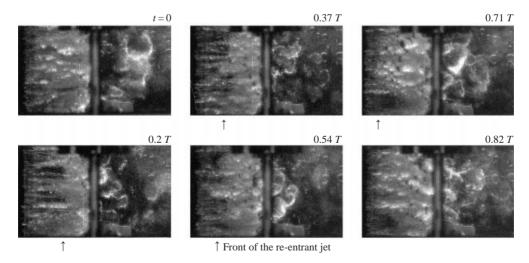
FIGURE 10. Visualization of the case of thin cavities (domain 2). Flow velocity  $11.6\,\mathrm{m\,s^{-1}}$ , confinement height  $e=20\,\mathrm{mm}$ , step height  $h=0.8\,\mathrm{mm}$ , divergence angle  $4.2^\circ$ . The period of the oscillation is 36 ms. The flow is from left to right.
