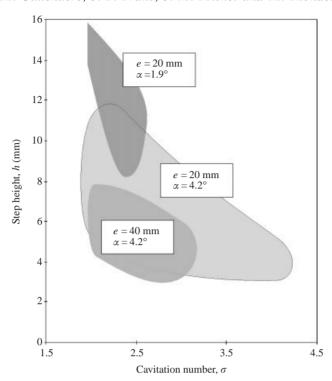
Figure 13. Evolution of the extent of cloud cavitation for different operating conditions at a flow velocity of  $11.6 \,\mathrm{m\,s^{-1}}$ .
